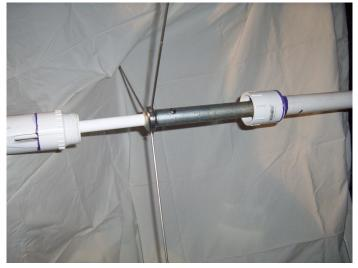
The new base mount is 1" water pipe-a lot tougher than that thin aluminum tubing. With the PVC armor extended down over the base mount, we can do without the guy lines at the antenna midpoint.
